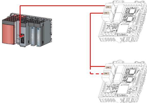
\*CC-LINK IE Field Option does not distinguish the directions of LINK1 and LINK2
