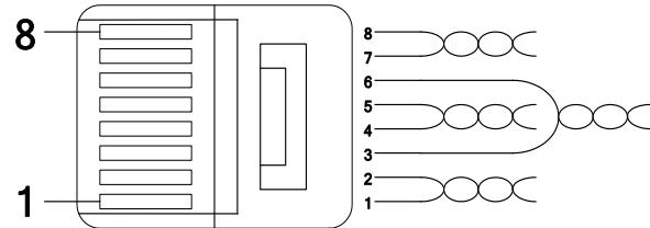
\*\* Wires connected to pin #1 and pin #2 must be twisted.
